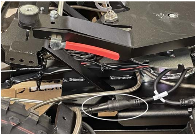
Figure 6.4.5 Location of the motor connector.
