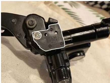
Figure 6.2.12 Location of the brake signal microswitch.
