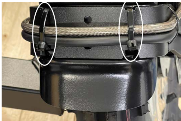
Figure 6.4.22 Detail of mudguard zip ties.
