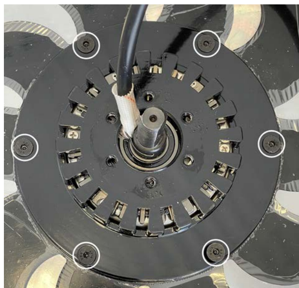
Figure 6.4.8 Location of screws holding the black wheel cover.
