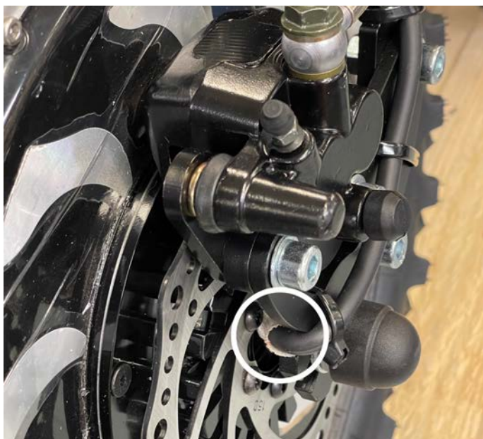
Figure 6.4.12 Correct routing of motor cable.
