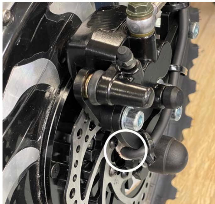
Figure 6.4.6 Correct routing of motor cable.
