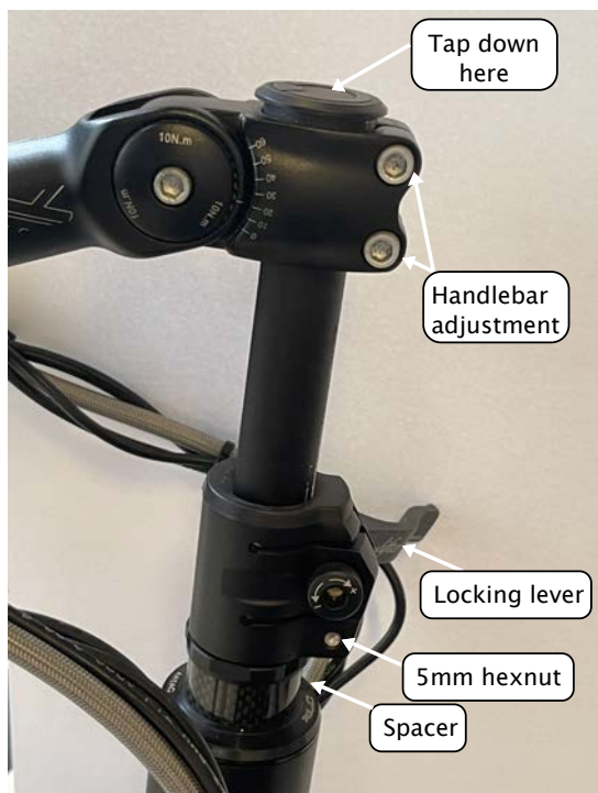
Figure 6.4.17 Steering column adjustment points.
