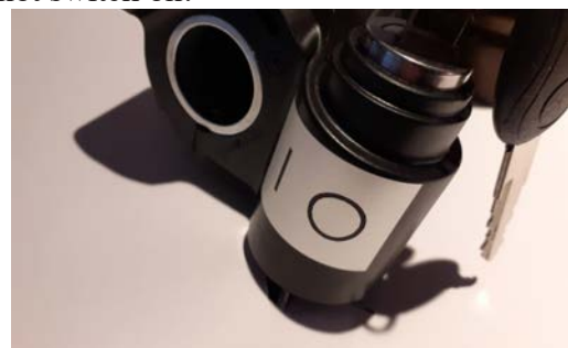
Figure 6.2.4 Throttle key switch markings 0=OFF / 1=ON.
