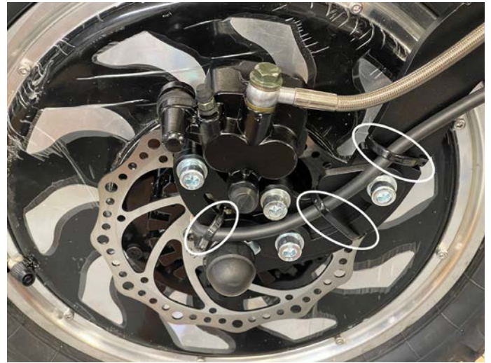
Figure 6.3.1 Location of cable ties for motor cable.
