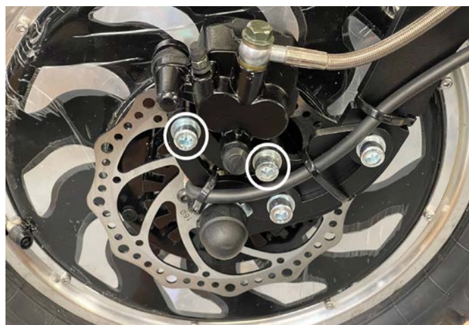
Figure 6.4.13 Brake calliper fastening bolts.
