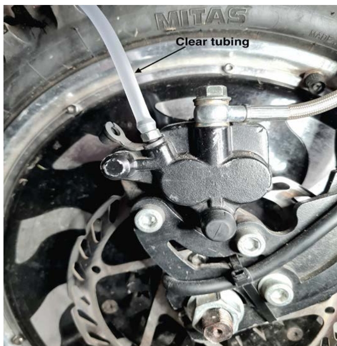
Figure 6.4.16 Clear tubing connected to the bleeder valve of the brake caliper.
