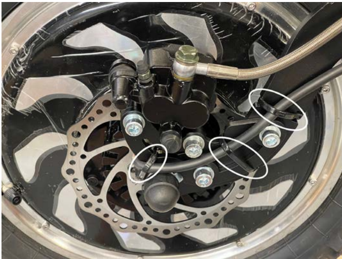
Figure 6.4.4 Location of cable ties for motor cable.
