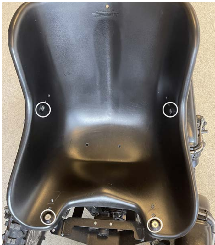
Figure 6.4.20 Location of the driver's seat fastening screws.
