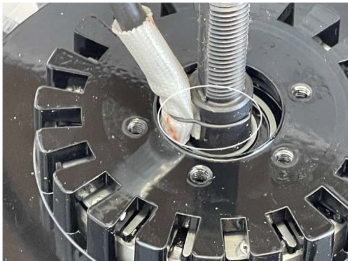
Figure 6.3.5 Location of motor cable attachment, in figure the clip version is shown.
