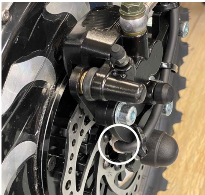
Figure 6.3.8 Correct routing of motor cable.
