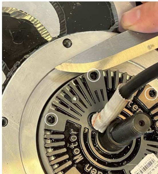
Figure 6.3.6 Example of how to facilitate removal of controller card housing with a knife.
