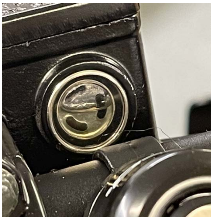
Figure 6.4.15 Master cylinder at 50% level.
