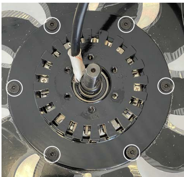
Figure 6.3.4 Location of screws holding the black wheel cover.
